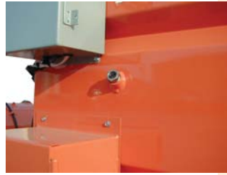
Above: The sight gauge located next to the control box, allows easy monitoring of flame.
