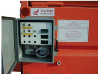
Above: The control box electronically controls up to three sources independently.
