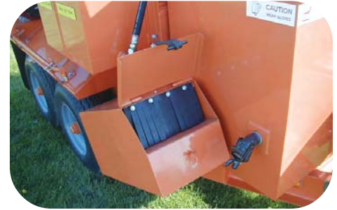
Shovel/Tool rinse storage tank option shown above.
