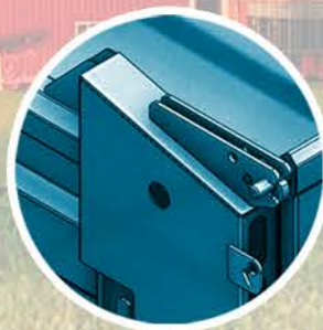
SIDE-SWING TAILGATE RELEASE HARDWARE
