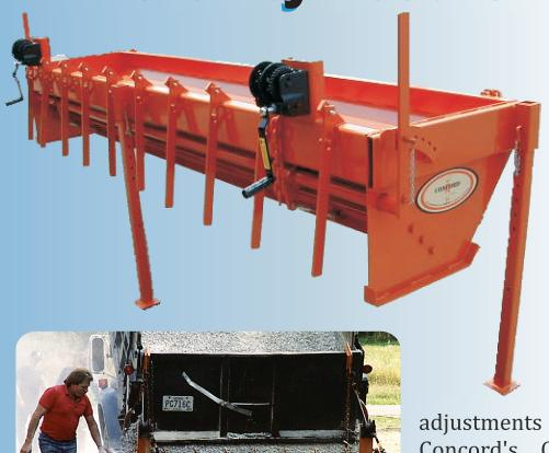
The Concord Gravity Feed Chip Spreader is a simple and cost effective machine for spreading all types of aggregate. This heavy duty deluxe spreader features a 1/4 inch thick rigid frame, and a one-piece sliding floor that is adjustable at either end of the unit in 1/2 inch increments to a maximum opening of 4 inches. Individually selectable sliding shutoff gates easily spread allow for width
