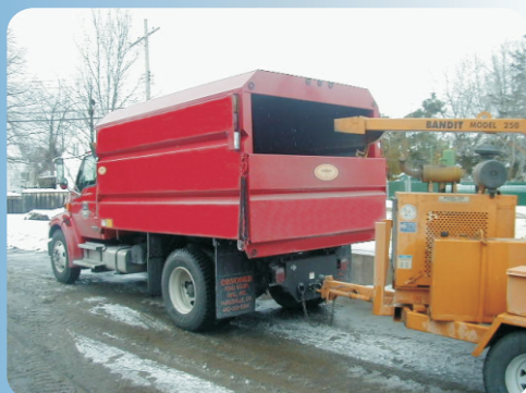
THE WCB 08-14 SERIES WOOD CHIP BOXES ARE AVAILABLE IN 8 FT, 10 FT, 12 FT AND 14 FT LENGTHS.
