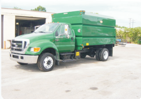
THE WCB 08-14 SERIES WOOD CHIP COLLECTION BOXES CAN BE MOUNTED INTO AN EXISTING DUMP BODY OR DIRECTLY TO THE CHASSIS.
