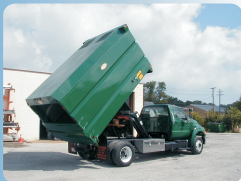
THE WCB 08-14 SERIES WOOD CHIP COLLECTION BOXES CAN BE MOUNTED INTO AN EXISTING DUMP BODY OR DIRECTLY TO THE CHASSIS.
