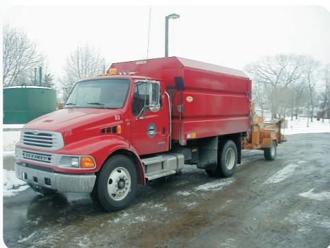
THE WCB 08-14 SERIES WOOD CHIP BOXES ARE AVAILABLE IN 8 FT, 10 FT, 12 FT AND 14 FT LENGTHS.
